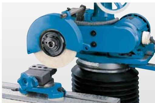
Surface grinder with angular adjustable vise
