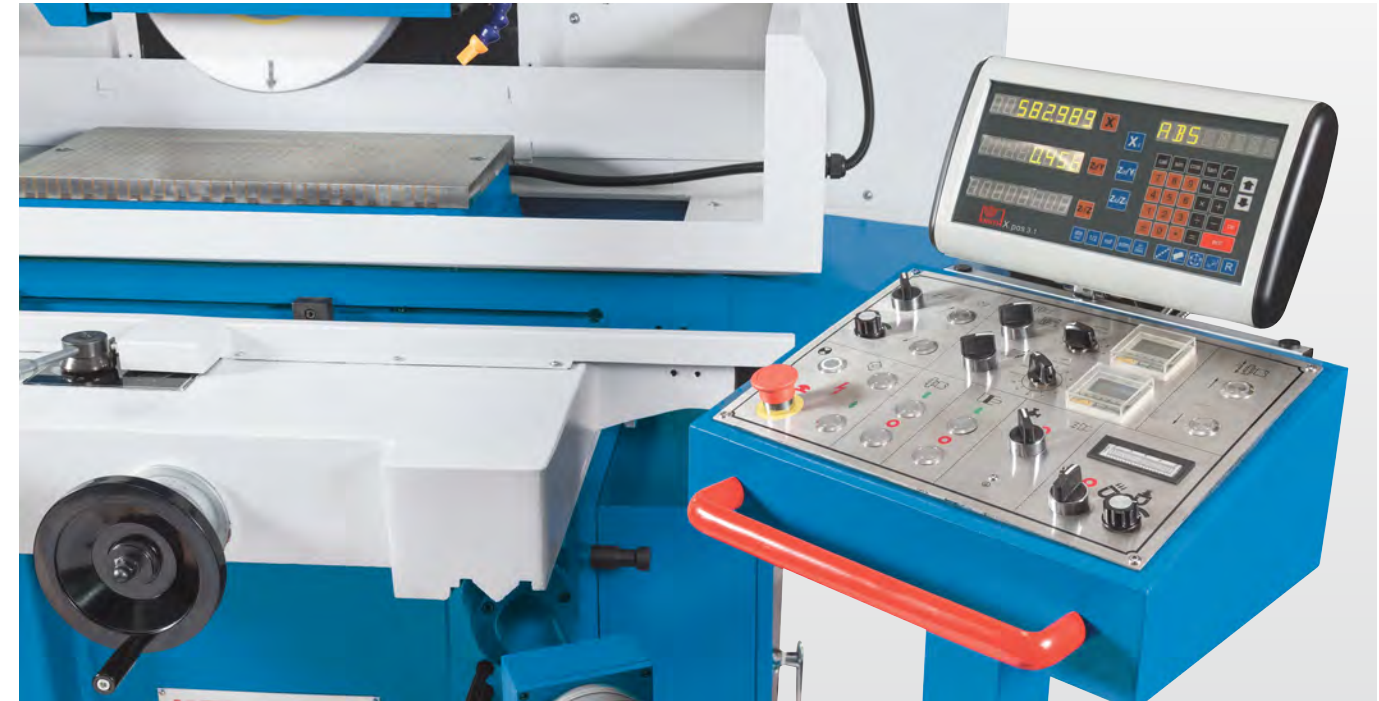
The standard position indicator ensures high precision and production safety
