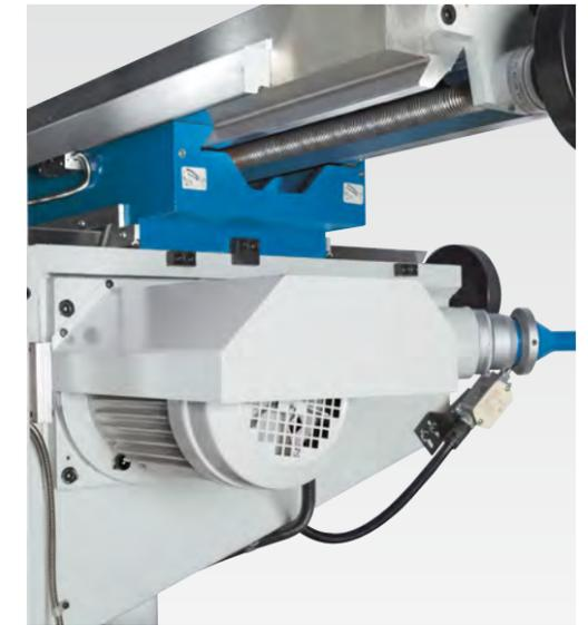
Rapid feed on Z axis with safety switch
