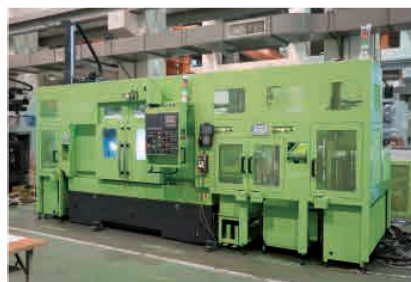
Single Machine + Single Robot Arm ( w /work-piece cleaning and detecting device )
