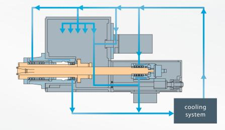
The spindle cooling system uses oil cooling and water jacket device to give the right amount of coolant to all the bearings, motors, gears inside the spindle box. This effectively reduces spindle thermal distortion and ensures working accuracy.
